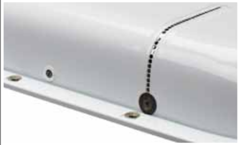
Low profile radome and ARINC 781 form factor allows for ease of maintenance on Air Transport platforms
